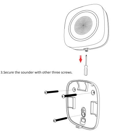
4. Fix the front panel on the sounder body. Tighten the set screw to complete the installation.
